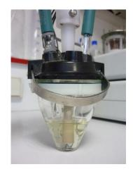
CAOX® is calculated with the integration of a voltammogram on a range of potentials, delimited by two distinct potentials.
